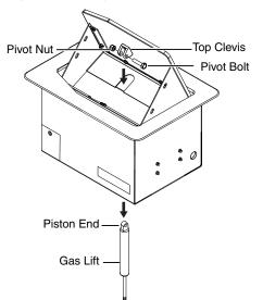
Figure 3-8 — Replacing the gas lift, HSA 200 model
